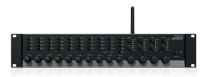
The PRE2xx series pre-amplifiers are solutions for applications where a large number (up to 8) of microphones (or other mono balanced audio inputs) need to be mixed to two (PRE220) or four (PRE240) output zones. The multifunctional stereo design with a total of 10 inputs allows connection for any type of audio source such as microphones, Bluetooth devices or line level audio sources.
