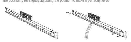
Make sure the appropriate fasteners are used, depending on the mounting surface (brick, concrete, wood, ... )
